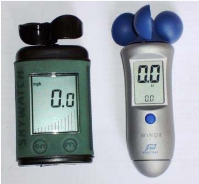
Figure 19: Two makes of digital cup anemometers with LCD displays
