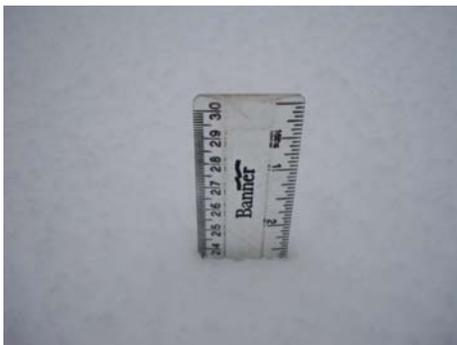
Figure 15. Depth of snow being measured with an ordinary ruler
