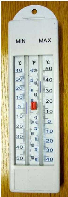
Figure 2: A maximum-minimum thermometer
