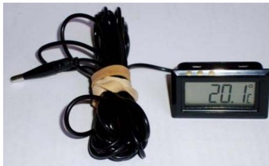
Figure 6: Digital thermometer with probe on a lead
