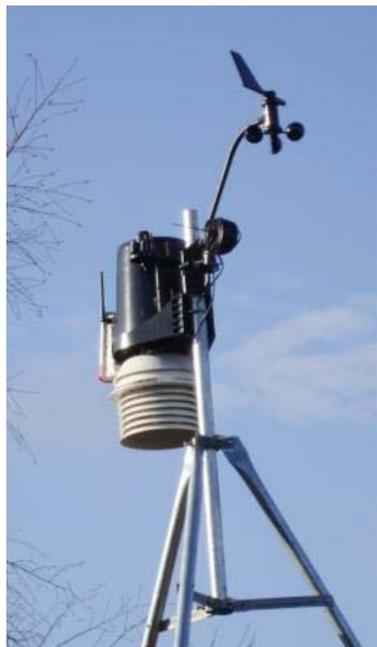
Figure 21: A wireless weather station measuring temperature, humidity, rainfall, wind speed, wind direction and pressure, transmitted to an indoors display unit.
